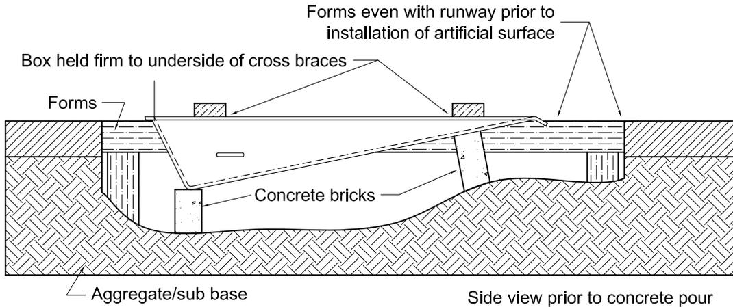
Dam concrete over slope to avoid a thin edge fill void when installing runway surface
