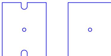
Each lid comes with two sets of captive covers. Each set consists of one notched cover for use with cables entering the box and one solid cover for use when the box is not in use.
